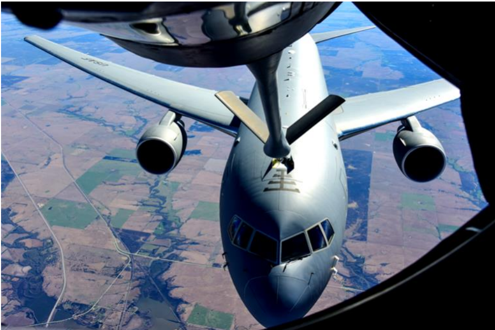
A KC-46A Pegasus from McConnell Air Force Base maneuvers into position to receive fuel from a KC-135 Stratotanker April 8, 2019, over Kansas. The KC-135 can transfer a maximum load of 200,000 pounds of fuel. (U.S. Air Force photo by Airman 1st Class Skyler Combs)
